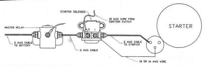
FOR MOST STARTERS, THE LIGHT GAGE (16 OR 18) WIRE CAN BE OMITTED. THE STARTER WILL HAVE A JUMPER BETWEEN THE SMALL CENTER TERMINAL AND THE LARGE TERMINAL WITH THE INCOMING VOLTAGE.
